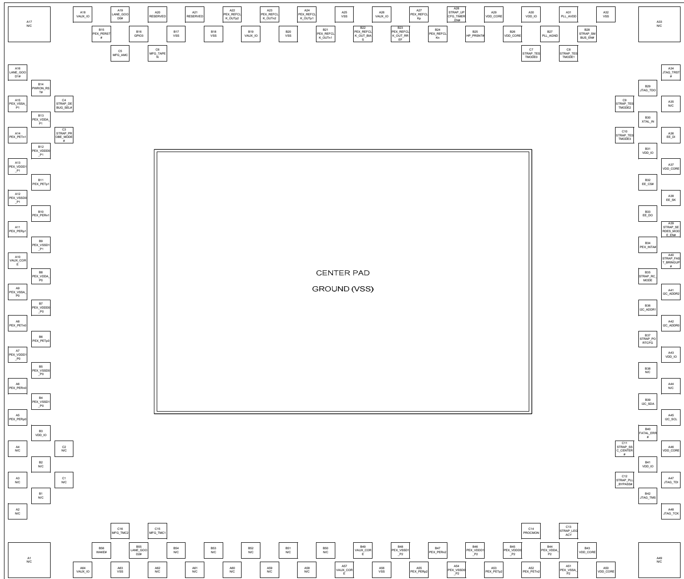
Figure 3-2. PEX 8603 Physical Signal Locations (Bottom View, as seen from Underside of Chip, 10 x 10 mm 2 Dual-Row aQFN Package)
