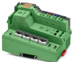
The modular Inline controller for automation applications in infrastructure, energy, and buildings is based on the Niagara Framework®. Four LAN, two USB, and two RS-485 interfaces as well as a LON interface (CEA-709) are integrated. The controller can be extended with numerous Inline I/O modules.
