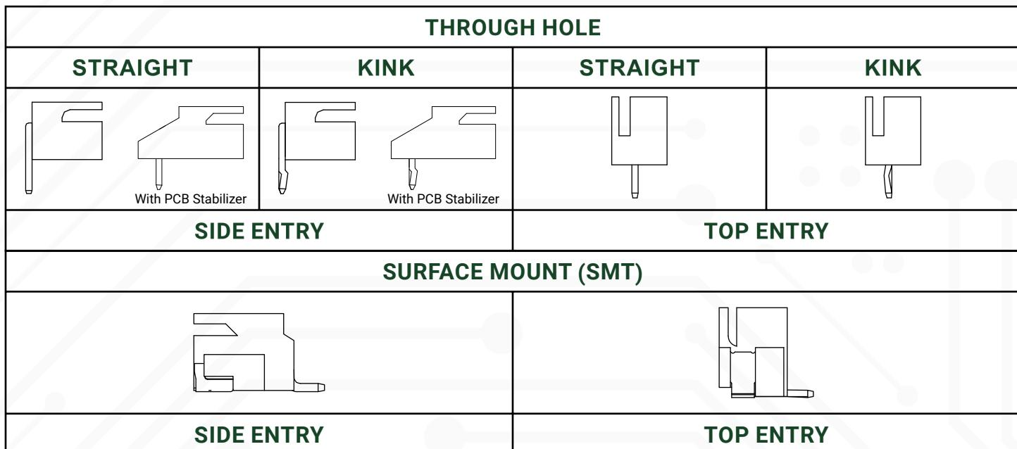
\* The above illustrations are for the male connector assemblies available. Male and female connector housings are also available and use crimp contacts. See [ordering guide](#) for details.
