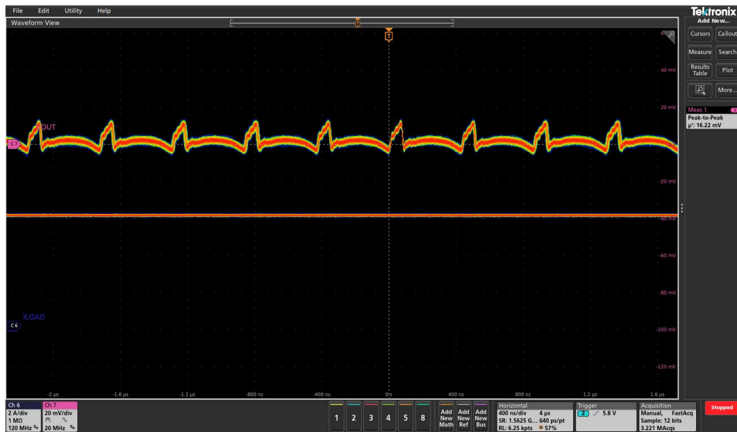
Figure 17 V_{OUT} ripple at 6A (Ch6:I o , Ch7:V OUT ), Peak-Peak V_{OUT} ripple = 16.2 mV
