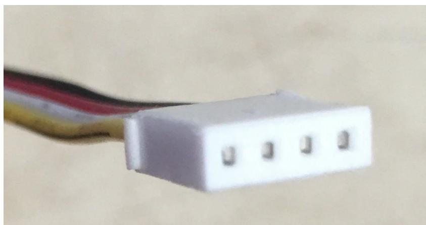
3. Once the tabs have been removed the connector can now be inserted into the NL-AB-RPI adapter upside down. The cable should be oriented so that the ground wire (black wire) is on the left side of the J9 or J10 connector on the NL-AB-RPI.
