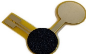
SEN0028 with NANOCOMP-CRC-10X10 material
