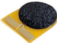
SEN0013 with NANOCOMP-CRC-10X10 material
