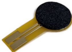
SEN0022 with NANOCOMP-CRC-10X10 material
