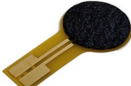
SEN0016 with NANOCOMP-CRC-10X10 material
