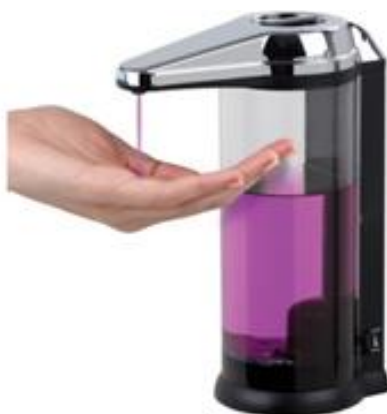
Figure 2-45. Proximity Sensing Based on CapSense in a Soap Dispenser
