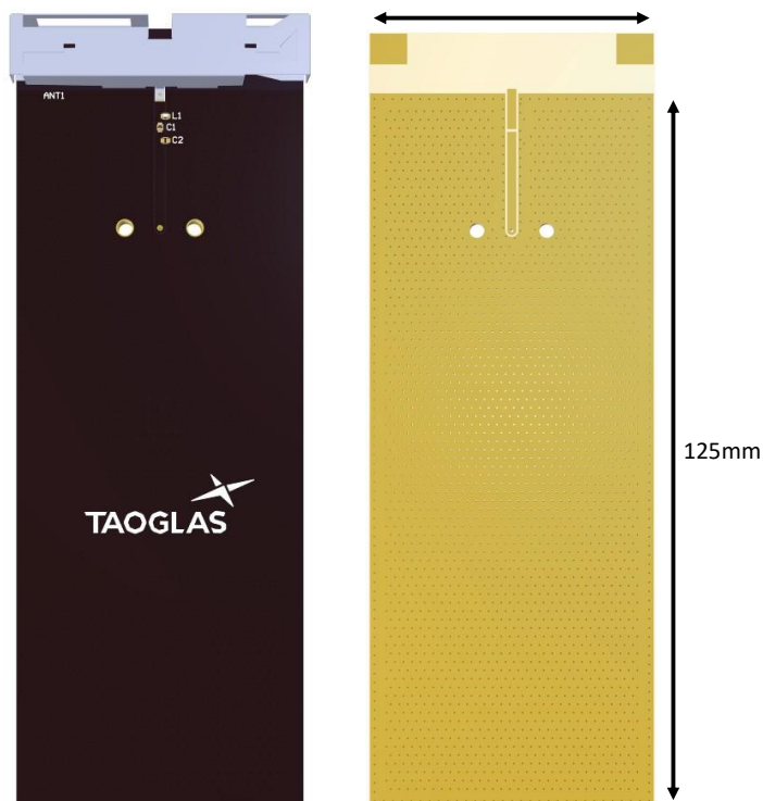
Top Side (MPA.66.A placement on 50x125mm PCB)
