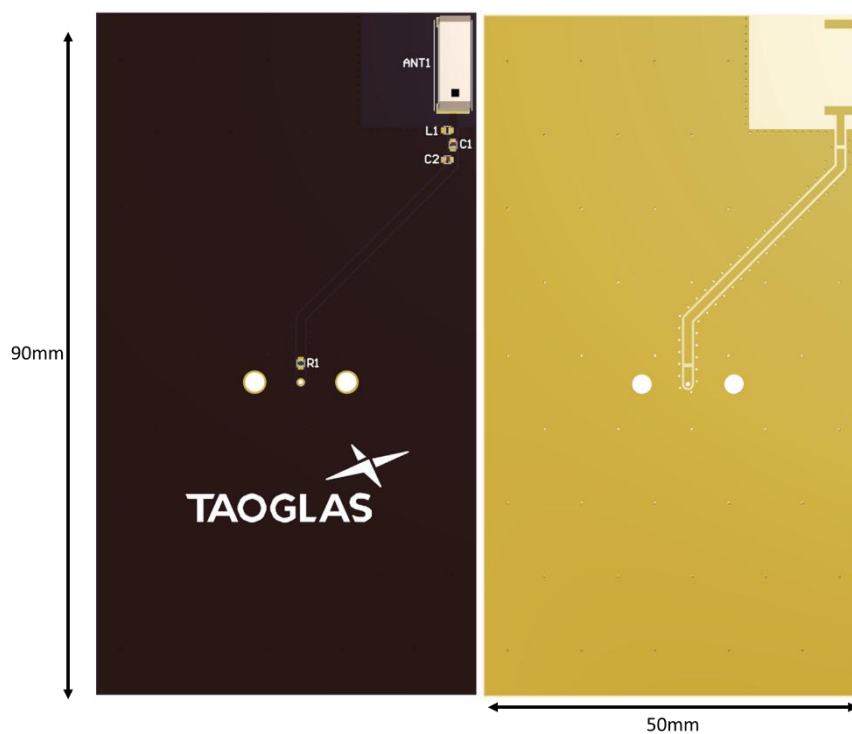
Top Side (ILA.89 placement on 90x50mm PCB reference design)
