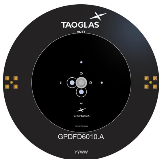
Top Side (GPDF6010.A placement on 70x70mm PCB)
