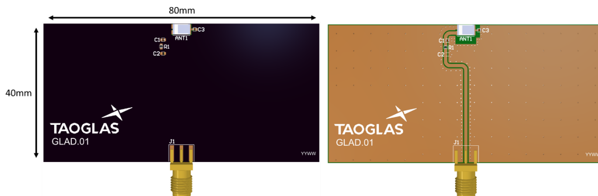
Top Side (GLA.01 placement on 80x40mm PCB reference design)
