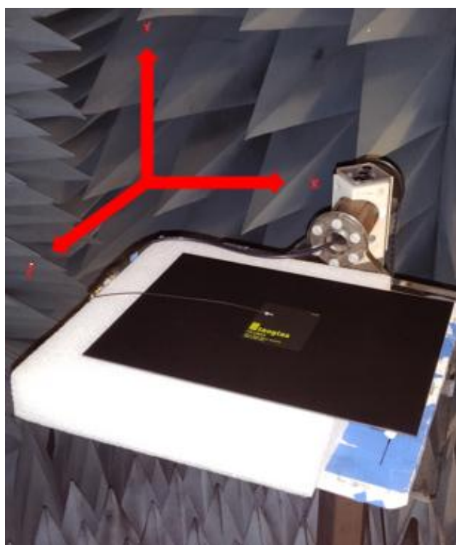
Chamber Test Set-up on 2mm ABS
