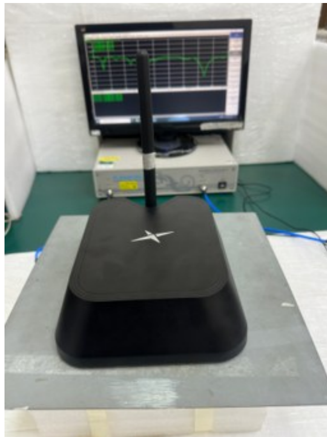
VNA Test Setup – Tested on the Patriot Antenna mounted on a 30x30cm Ground Plane
