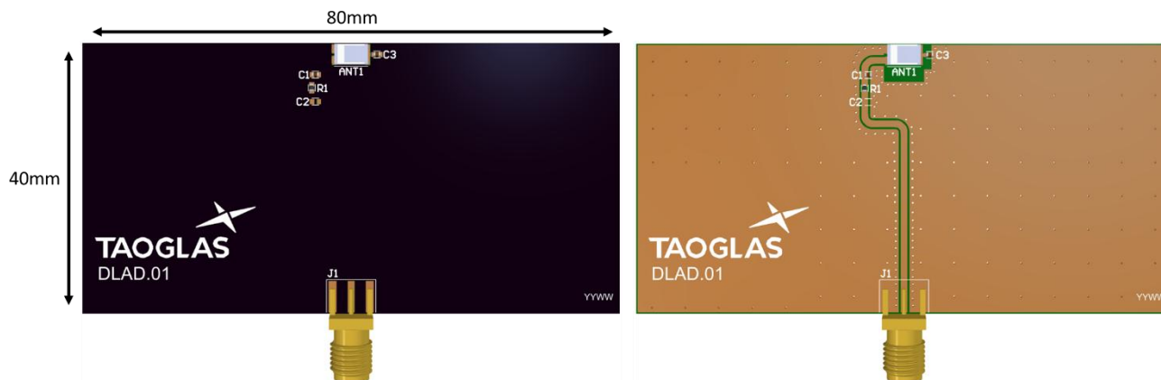
Top Side (DLA.01 placement on 80x40mm PCB)
