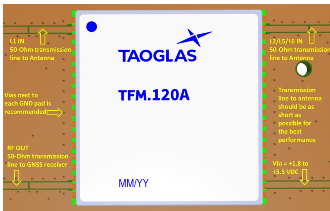
TFM.120A module mounted on a PCB, showing transmission lines and integration notes.
