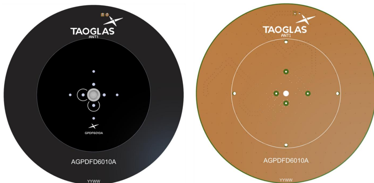
Top Side ( GPDF6010.A placement on 70x70mm PCB)
