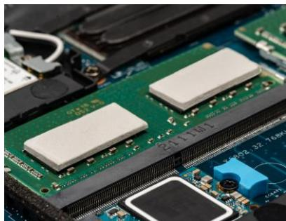
Tflex™ SF16 is an innovative, ultra-high performing thermal material in Laird's gap filler portfolio. This non-silicone material measures 16 W/m•K in thermal conductivity and has excellent deflection properties which provides minimal pressure on components during deflection. Very little pressure is required to reach the lowest possible thermal resistance.
