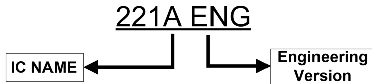
Figure 9.1: IQS211A Engineer Version, Marked as 221A
