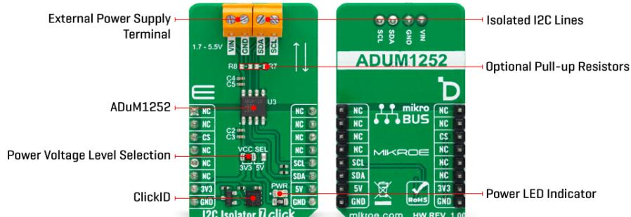
I2C Isolator 7 Click uses a standard 2-Wire I2C interface to allow the host MCU to have an isolated bidirectional data transfer with a connected I2C device to the I2C terminals. As we mentioned, besides the I2C bus, the power supply is isolated, too. Places for optional pull-ups on the I2C bus are left unpopulated. You can solder resistors according to your needs.
