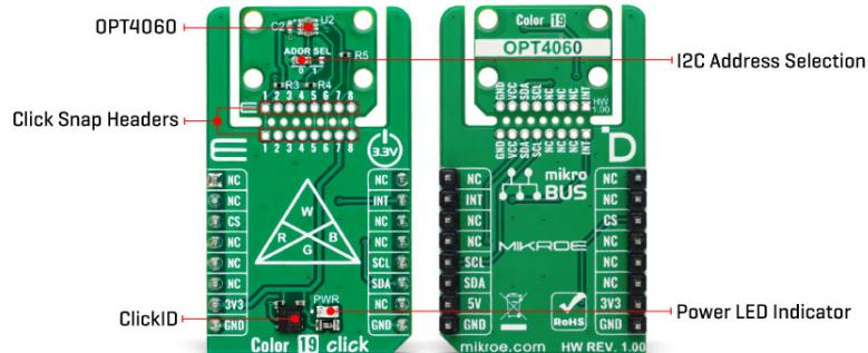
The OPT4060 incorporates specialized optical filters with finely tuned spectral responses for the RGB channels. This ensures strong rejection of wavelengths outside their target range, particularly in the near-infrared (NIR) spectrum at 850 and 940nm. This ensures reliable measurements in environments where NIR interference is prevalent. Additionally, its wide-band channel provides comprehensive light intensity data, allowing for precise lux calculations and color characterization.
