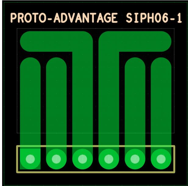
Shown with 1.27mm grid. Traces are 2.00mm width. Air gap between traces is 0.54mm.
