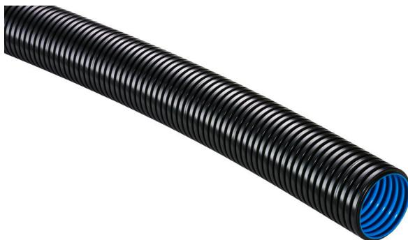
Highly flexible conduit for robotic applications with a unique wear indicator function. Especially suitable for narrow bending radii and high abrasion
