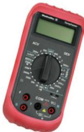
Multimeters are capable of measuring a number of variables. Each instrument can measure voltage and resistance, as well as performing continuity and diode testing as standard.
