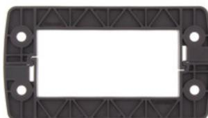
The frame, fabricated from a single piece, is quick and easy to assemble and consists of dimensionally stable, fibre-glass reinforced plastic. The captive foamed seal guarantees effective IP66 sealing in accordance with DIN EN 60529, even on painted and rough surfaces.
