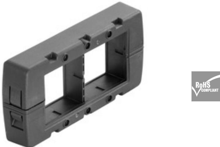
The frame, fabricated from a single piece, is quick and easy to assemble and consists of dimensionally stable, fibre-glass reinforced plastic. The captive foamed seal guarantees effective IP66 sealing in accordance with DIN EN 60529, even on painted and rough surfaces.
