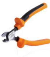
Cutting tools for conductors up to 8 mm, 12 mm, 14 mm and 22 mm outside diameter. The special blade geometry allows pinch-free cutting of copper and aluminium conductors with minimum physical effort. The cutting tools (KT 8 to KT 22) also come with VDE and GS-tested protective insulation up to 1,000 V in accordance with EN/IEC 60900.
