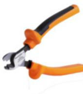
Cutting tools for conductors up to 8 mm, 12 mm, 14 mm and 22 mm outside diameter. The special blade geometry allows pinch-free cutting of copper and aluminium conductors with minimum physical effort. The cutting tools (KT 8 to KT 22) also come with VDE and GS-tested protective insulation up to 1,000 V in accordance with EN/IEC 60900.
