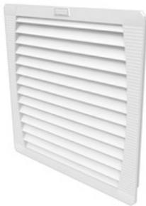
The fluted filter mat of the IP 55 version extends the service life by up to 300% in comparison to conventional filter mats. Thought out details as the functional flap cover enable a fast and tool-less change of the filter mats which saves time and money.
