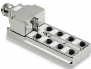
Some applications require complete shielding from the sensor to the control. Our metal SAI distributors achieve this complete shielding. EMC glands are included with the distributors. Initiator LEDs are omitted.
