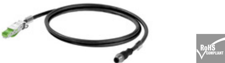
Assembled IE lines, railway cable RW (reduced wire), cat. 5, PUR, black, RJ45 plug, no tools required, IP20 and M12 straight pin
