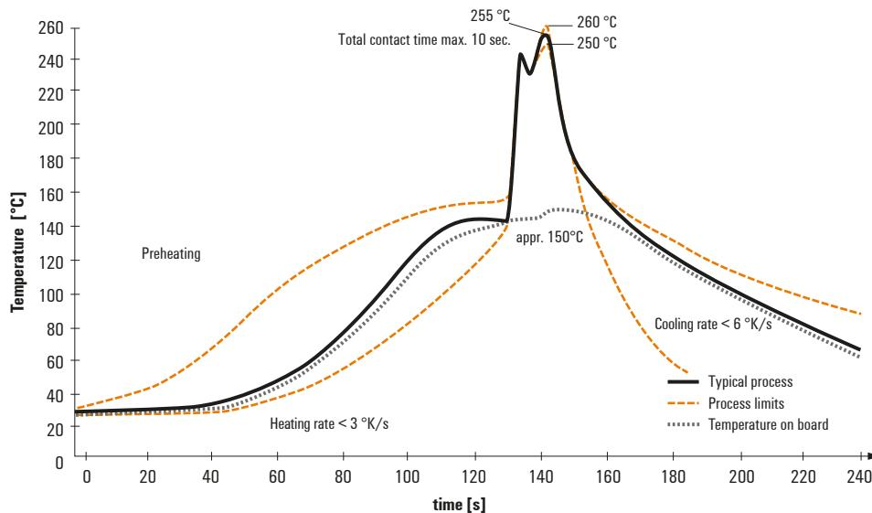
**Wave soldering profiles**
