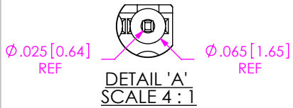
FIG 3 *SD1: SOLDER DONUT (ONE PER POSITION) (ROW STYLE -S,-D,-T & -Q ONLY) *NOT ENGINEERING APPROVED
