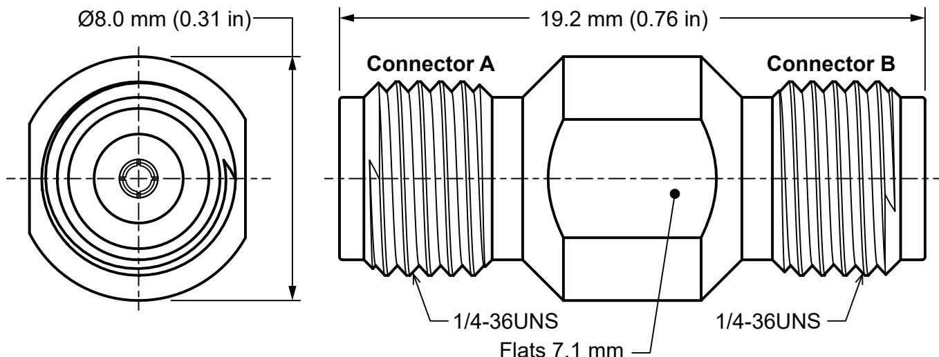
Figure 1: Product Dimensions for the ADP-2.92F-2.92F Adapter
