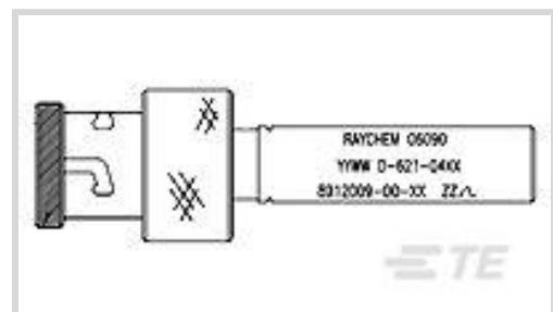
Contact Type: **Pin**Impedance: **78 Ω**Data Bus Connector Style: **Bayonet**Data Bus Connector Type: **Plug**Polarization Code: **D**
