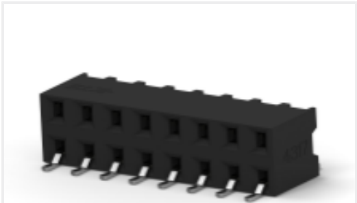
TE Part #1-2307729-6 16P,2MM,B-B,REC,DRHZ,SMD,0.1AU,TR
