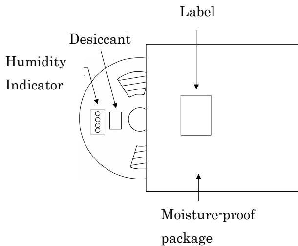
Reel will be packed in moisture-proof package together with desiccant and humidity indicator.
