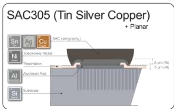
Figure 6 – Top electrode description of SAC305 pre-bumped version
