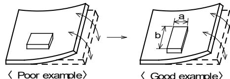
(2) Components location on PCB separation
