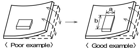
(2) Components location on PCB separation
