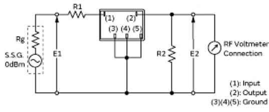
$R_g + R_1 = R_2 = \text{Input/Output Impedance}$
