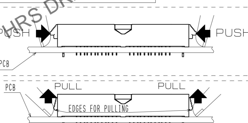
Pull up the front lever and the edges of lock levers of the plug vertically at the same time, catching and pushing the edges of lock levers with finger at the both sides
