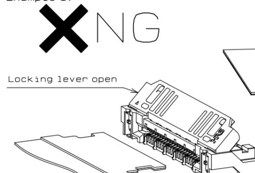
Align both sides of FPC horizontally to the sides of the connector opening and insert straightforward.
