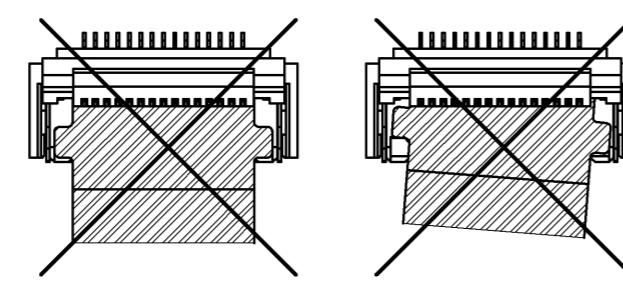
◆ Checking the Locking Condition
