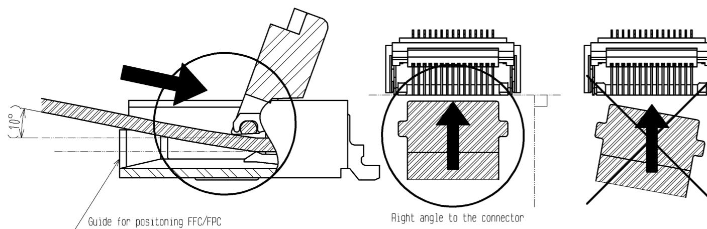
2. Do not insert the FFC/FPC diagonally from above.
