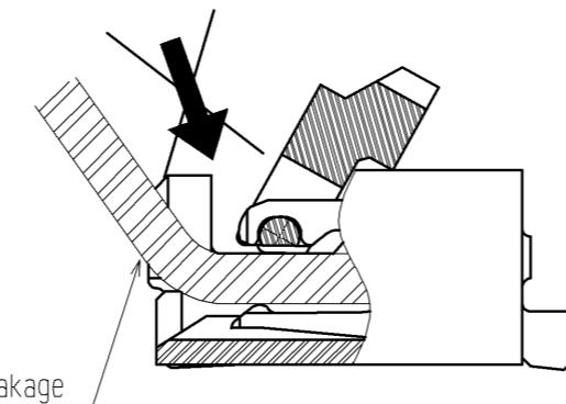
◆ Checking the Locking Condition
