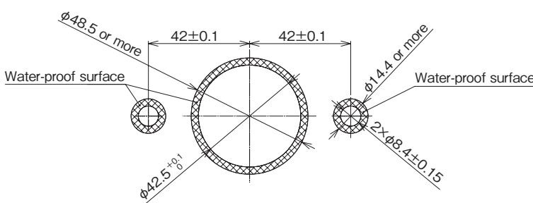
Recommended panel thickness  $t=2$  to 4.5mm
