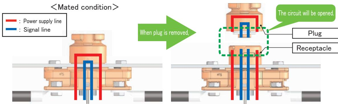
When the connector is unmated, the circuit is physically disconnected, ensuring the safety of workers.
