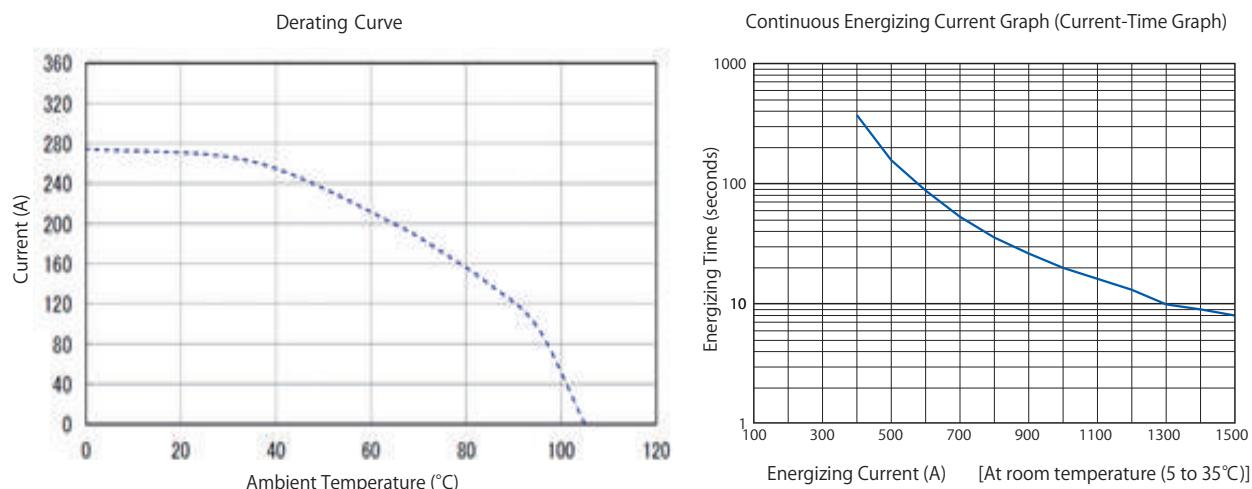
Operation below the derating curve (dotted line) is recommended.
