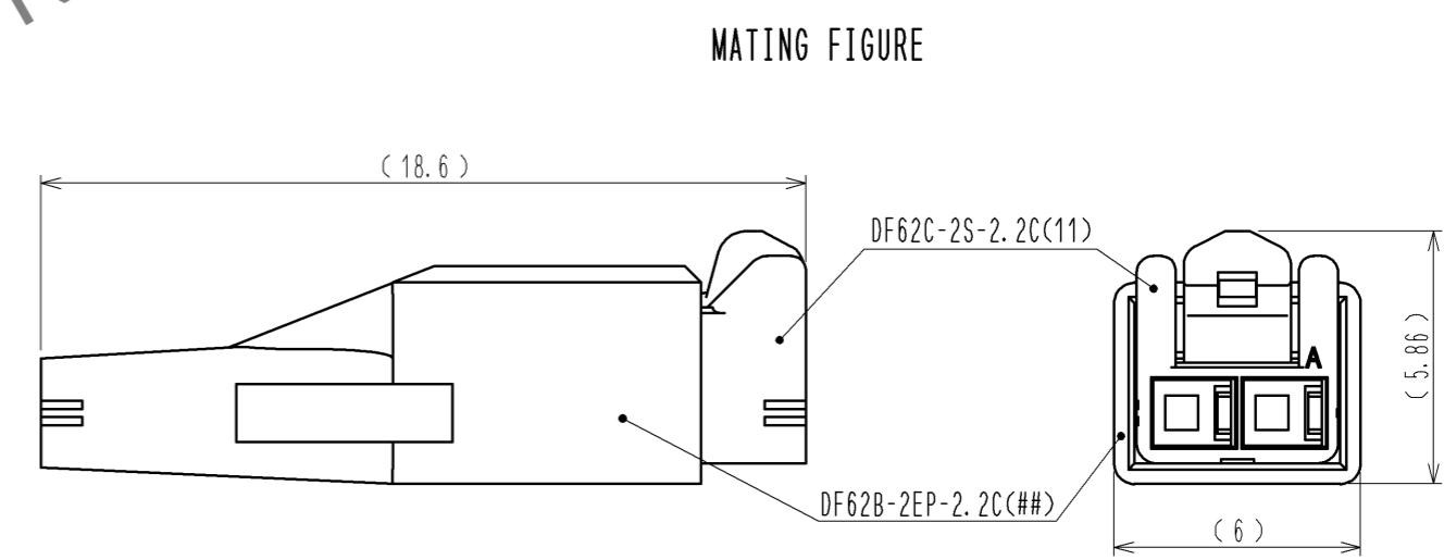
NOTE. ①> MARKINGS AT THE INDICATED POSITIONS ARE CONTACT NO. MARKING. AND SHAPES ARE SHOWN IN FIGURE-1.
