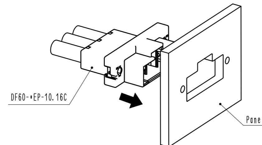
2. Tighten a screw (Size:M3) to fix with panel.
