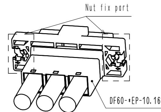
1. Slide a nut (Size:M3) to nut fix part.
