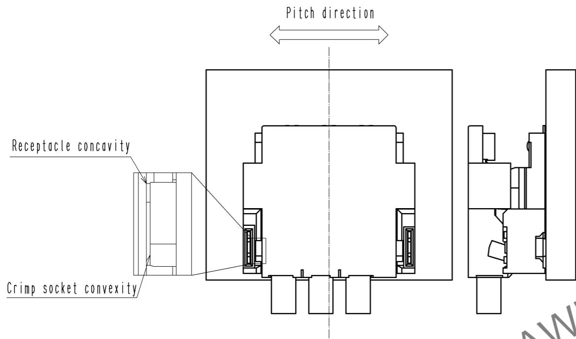
2. Keep pressing down at the cable side and also apply force to the lever side to mate.
