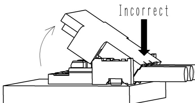
Make sure to use the lever for removal operation.
