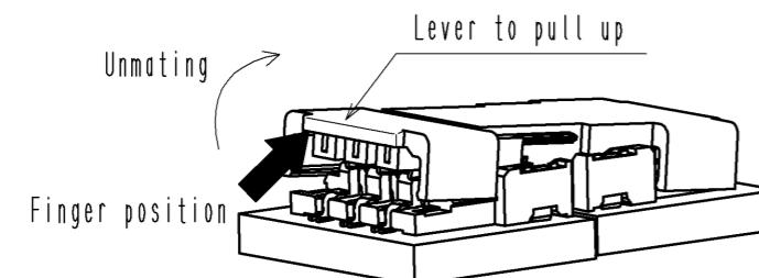
2. After releasing either side, hook the lever on the other side with a finger and lift up to the upper direction, too.
