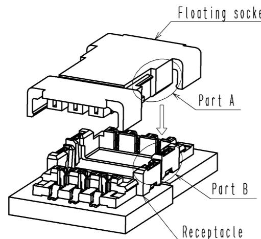
2. Align the floating socket edge on the side of friction lock to receptacle housing edge in a line.
