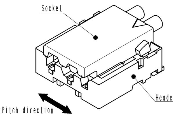
②Slightly press the socket down at cable side to tilted angle.
