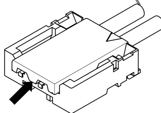
②Lift up to the upper direction and friction lock is released.
