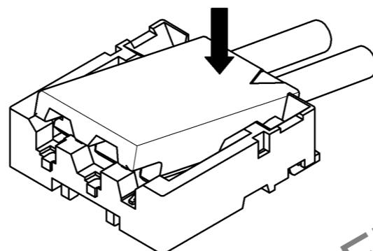
③Press down at the lever side with stabilizing the cable side to insert. Mating completes.
