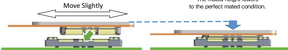
3. In the engaged state, the connectors are parallel to each other, and the connectors cannot move forward, backward, left, or right. Complete mating from this state.
