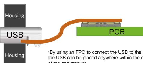
\*By using an FPC to connect the USB to the PCB, the USB can be placed anywhere within the design of the end product.
