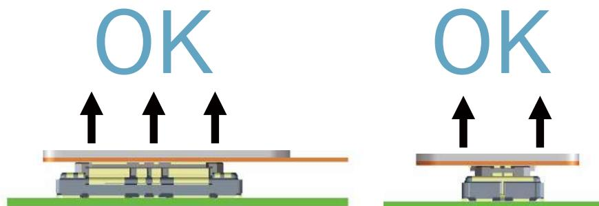
2. If difficult to remove, extract the connector diagonally in the direction of the pitch.
