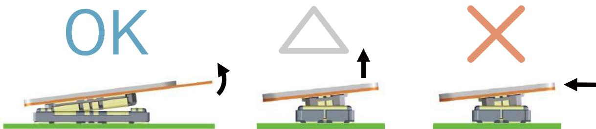
3. If the FPC does not have sufficient rigidity, solder stripping or connector breakage may occur.
